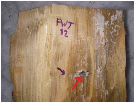
FIGURE 12 Section of the stem taken from Tree #12 (ponderosa pine) showing white mycelial filaments and brown cubical decay in the heartwood surrounding the drill hole (at red arrow). Note that the inoculant dowel is no longer present and that extensive sap rot is also evident.
