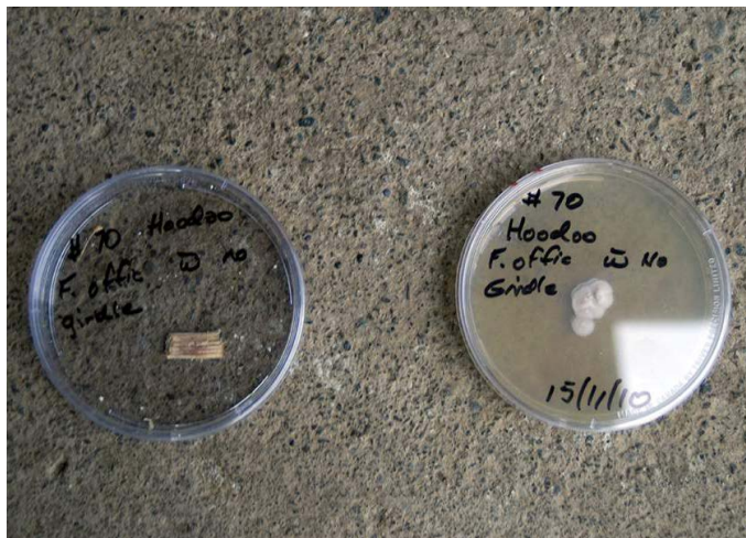
FIGURE 10 Wood sample taken from Tree #70 near the original point of inoculation with Fomitopsis officinalis (left); the same fungus re-isolated as a pure culture on growth medium in the laboratory (right).
