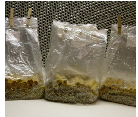
FIGURE 4 Fungi being established on wooden dowels inside sterile bags in the laboratory.
