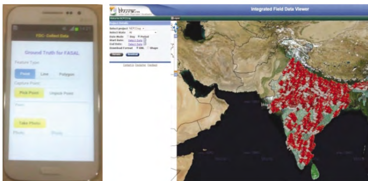
Figure 3. Real time ground truth collection using smart phone, a) Android app developed by NRSC, b) Ground Truth sites available on Bhuvan server
