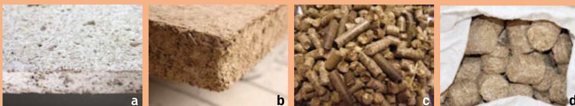
Products developed from reed biomass ( Phragmites australis ). a: fire resistant panel, (photo: Christian Schröder); b: construction board with reed fibres and clay (photo: Nina Körner), c: pellets (photo: Tobias Dahms); d: briquettes (photo: Nina Körner).
