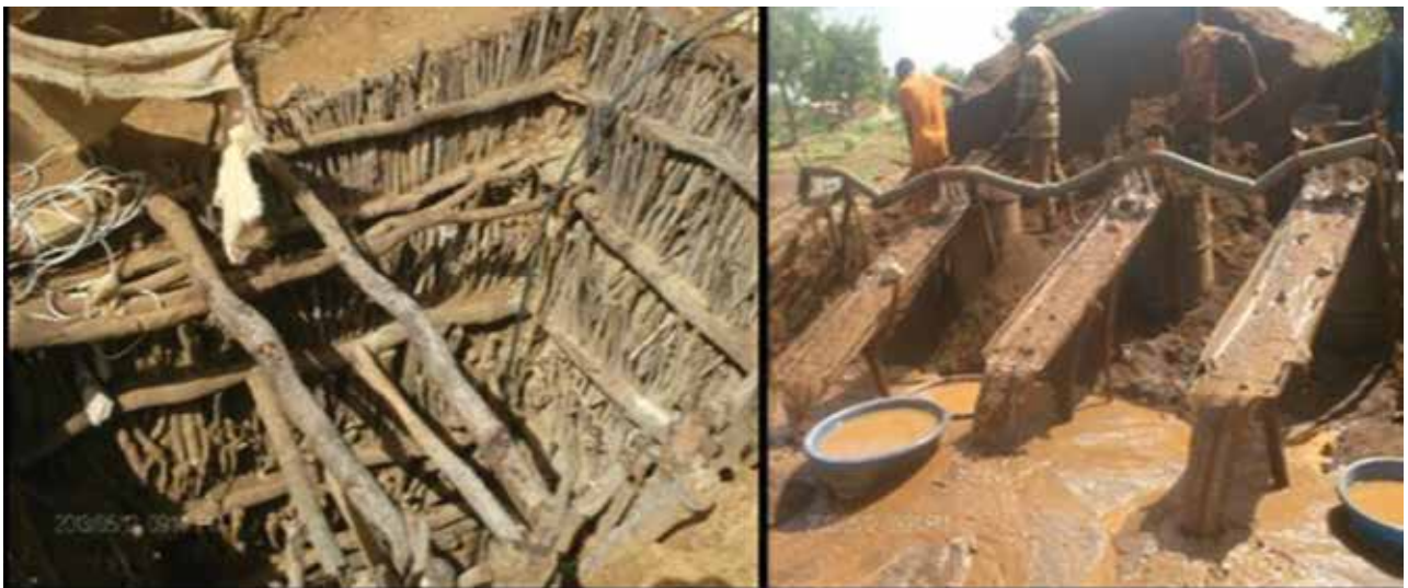
Figure 7. Pit wall blocking with forestays. Washing on long toms.
