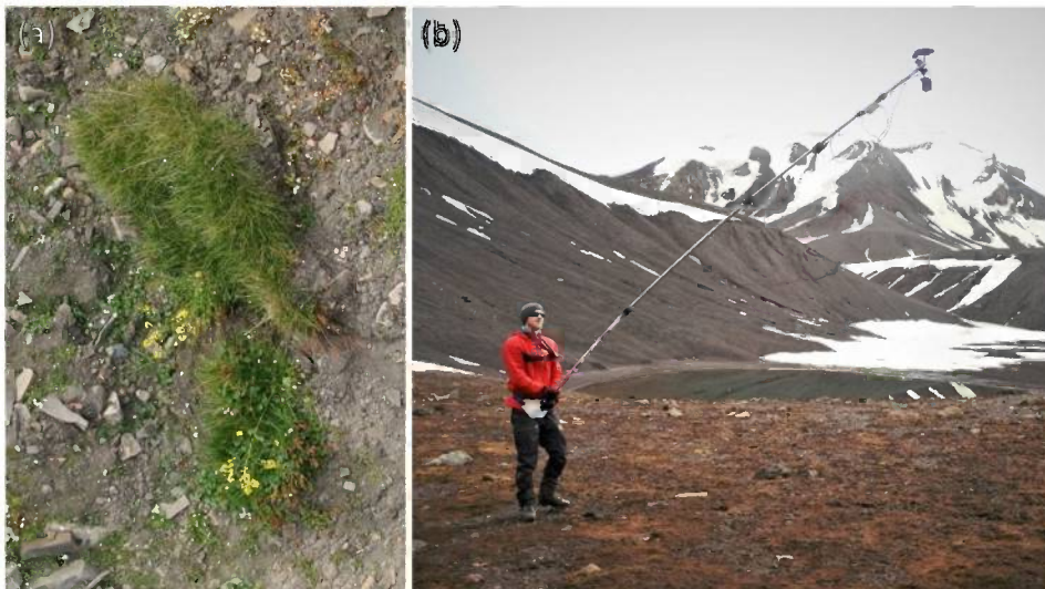
FIGURE 4 (a) Barbarea vulgaris in Barentsburg in 2019, as viewed from 4 m above ground altitude as an example for the HI photogrammetry resolution (photo: F. Wilken). (b) Example of the suggested manual photogrammetry set up (photo: D. Wasner)
