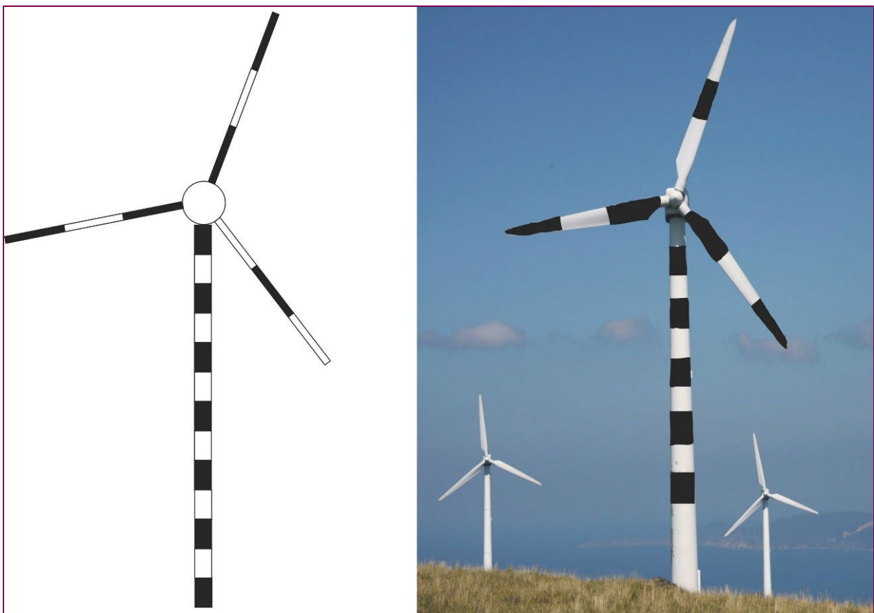
Figure 1: Illustration of high contrast blade markings. Left: diagrammatic indication of high contrast blade and pylon markings. Right: impression of markings applied to a turbine. Blades are divided into equal length black or white sections each one third the length of blade. The pylon is divided into equal length black or white sections each one half the length of the blade sections. N.B. Any final design or prototype would need to be compliant with regulations applying to marine structures, e.g., potentially painting the tips of individual blades red in accordance with Civil Aviation Authority, CAA guidance. Source: G R Martin, 2022. © 2022, G R Martin.
