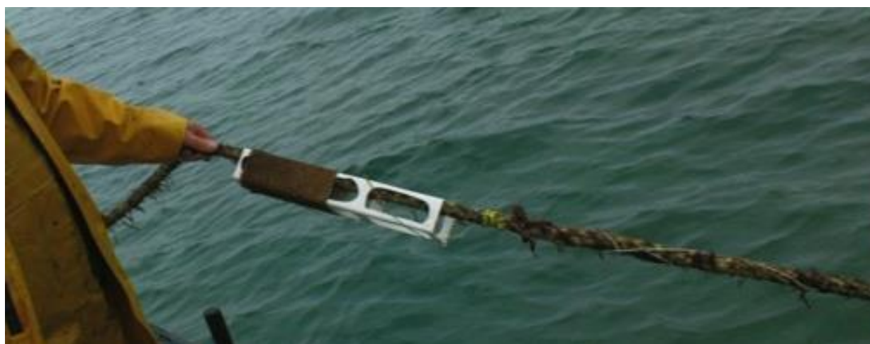
Figure 6 A spool of twine being deployed around a cultivation long line at sea. © Benoît Quéguineur. Reproduced with permission.
